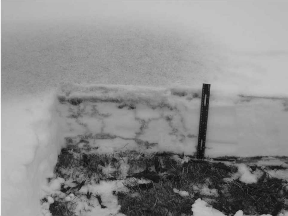
Figure 3.13 Flow fingers for preferential liquid-water movement that formed during initial day's melting of a homogeneous 28-cm depth snowpack resulting from a single snowfall in Pennsylvania (photo D. R. DeWalle). Water mixed with food coloring was uniformly sprayed over the snowpack surface to trace water movement. Also note evidence of meltwater movement downslope to the right in the surface layer and at the soil–snow interface. See also color plate.
