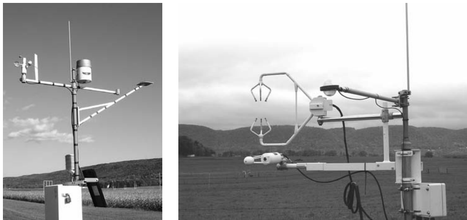
Figure 6.5 Solar-powered climate stations equipped with data loggers (left) are used to provide data (wind speed, air temperature, humidity) to support computations of snowpack convective exchange. The addition to climate stations of sonic anemometers (top right), fine-wire thermocouples, and high-speed open-path gas analyzers for \text{CO}_2 and water vapor (bottom right) allows computation of convective exchange using the eddy covariance method (photographs by D. DeWalle). See also color plate.
